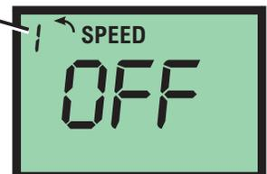
With pump operating in manual mode (Mode 1), pump speed can be changed at anytime by using UP or DOWN arrows during operation.
