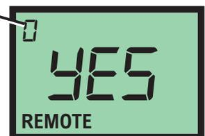
Running pump with Remote Start / Stop enabled, 'REMOTE' icon will always be visible on lower left side of screen. Pump will display 'STBY' (standby) if pump is in stop mode via contact closure signal. **Please use caution in this mode, pump can start at anytime. If you must perform maintenance to pump, press and release STOP button.**
