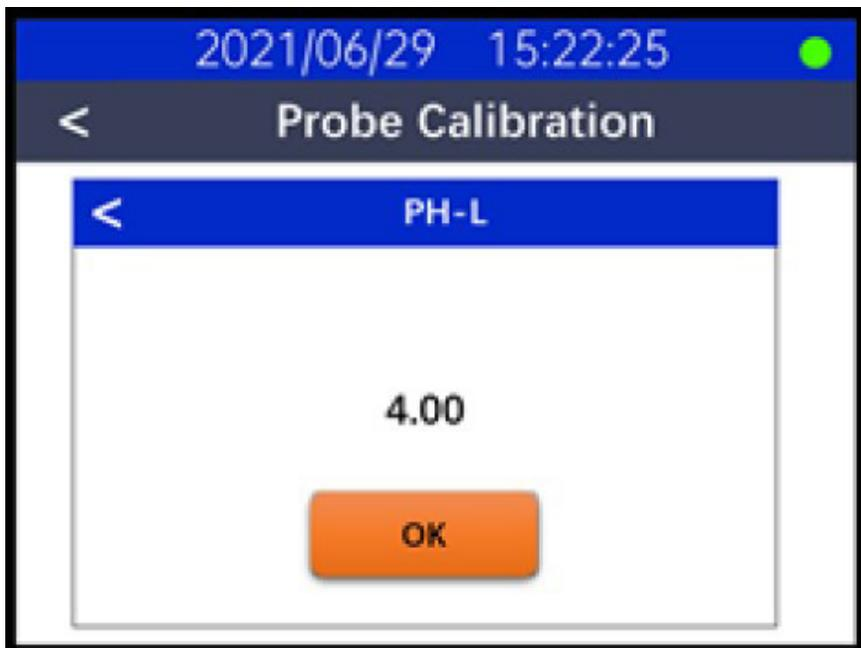
Select the Enter button on the probe confirmation page. The controller will then perform a calibration for the probe, and will wait for the calibration result. The probe calibration result will be automatically displayed on the calibration interface.
