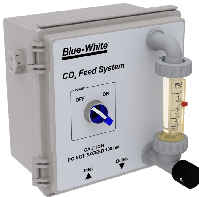
Figure 1. The Blue-White® CO 2 feed system maintains commercial swimming pool pH levels by directly injecting carbon dioxide into the water supply to create carbonic acid. This lowers the water's pH level naturally without hazardous chemicals such as muriatic acid or sulfuric acid. Flow is adjusted via the Blue-White® F-440 adjustable flow meter for accurate and consistent pH control.
