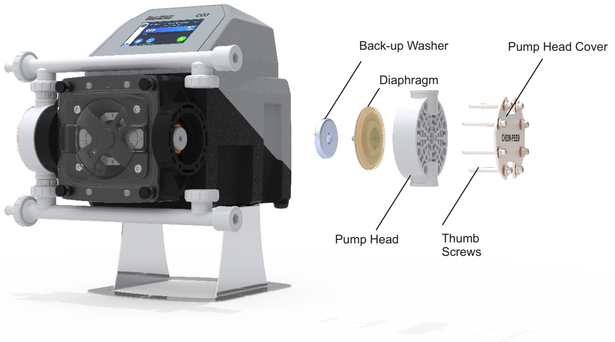
Pump Head and Diaphragm
