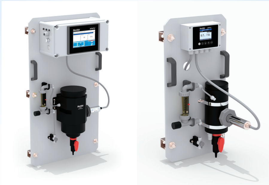
Figure 1 & 2. Instrumentation such as turbidity analyzers (left) and chlorine analyzers (right) are key to ensuring pre-treatment processes in direct potable reuse are working as required. Such instruments can communicate directly with chemical metering pumps in order to correct water quality when parameters are too far out of tolerance for the quality level desired.
