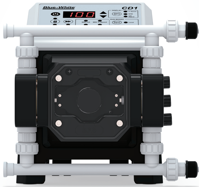
Figure 1. Multi-diaphragm pumps like Blue-White's CD1 operate so that when the first diaphragm is in the suction phase, the second diaphragm is in the discharge phase. The dual diaphragm design allows fluid to be pumped at a near continuous flow, creating a smooth chemical feed profile that minimizes the risk of vapor lock when dosing off-gassing chemicals, such as chlorine and PAA.
