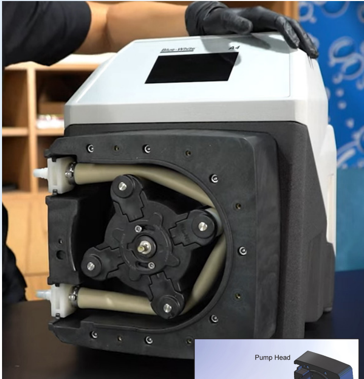
Figure 3. Peristaltic Pump Tubes
