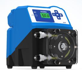
FLEXFLO's safety features include a built-in Tube Failure Detection System (TFD) and a lockout feature. The TFD system detects a tube rupture, automatically shuts down the pump to prevent chemical spills, and warns the operator of trouble. The safety lockout feature prevents unwanted tampering.
