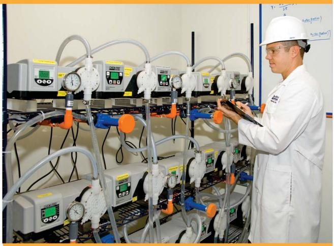
Extreme pressure and longevity testing for thousands of hours
