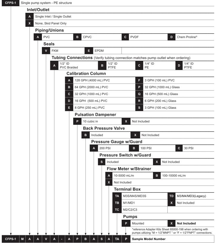
**NOTE:** When ordering pumps for skids, pump head orientation is standard LEFT facing only. All skids are pressure tested prior to shipment. Pumps are purchased and shipped separately. Contact factory for quote/pricing on 5-point performance testing. **Customer is responsible for ensuring skid components are compatible with any chemicals being used.**
