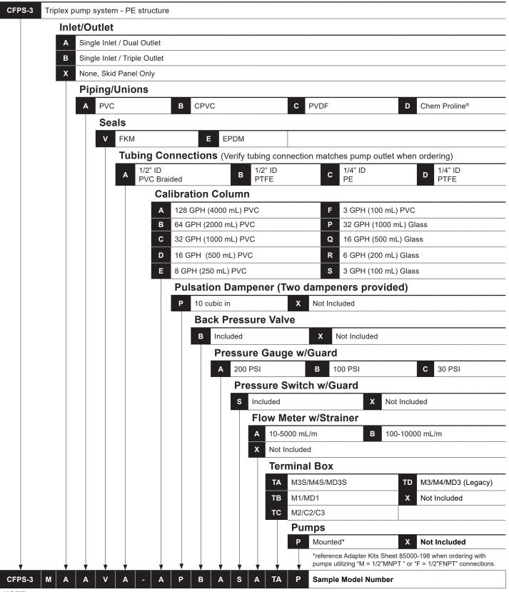
**NOTE:** When ordering pumps for skids, pump head orientation is standard LEFT facing only. When ordering skid with pumps of different model numbers, please include complete model number of each pump and location on skid with order. Contact factory for quote/pricing on 5-point performance testing. **Customer is responsible for ensuring skid components are compatible with any chemicals being used.**
