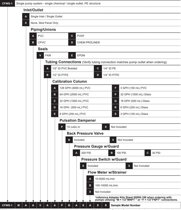
**NOTES:** When ordering pumps for skids, pump head orientation is standard LEFT facing only. Terminal Boxes quoted and mounted separately. All skids are pressure tested prior to shipment. Pumps are puchased and shipped separately. Contact factory for quote/pricing on 5-point performance testing. **Customer is responsible for ensuring skid components are compatible with any chemicals being used.**
